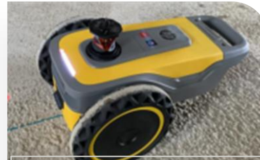
Marking robot for building construction
